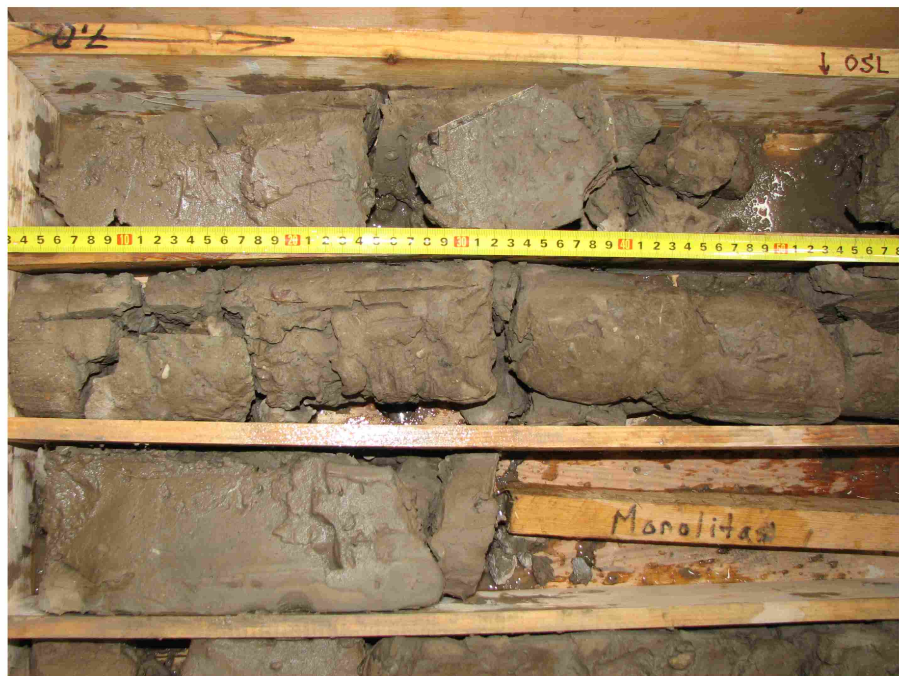
Fig. S4. Core of sampled grey-brown till in borehole 84.
