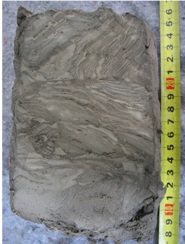
Fig. 6.4 Glacioidislocated inter-till sediments represented by deformed micro-layers of fine sand, silt and clay in the core of borehole 36888 (depth 33.5 m)
